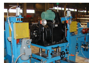
On line inspection of ERW tubes
